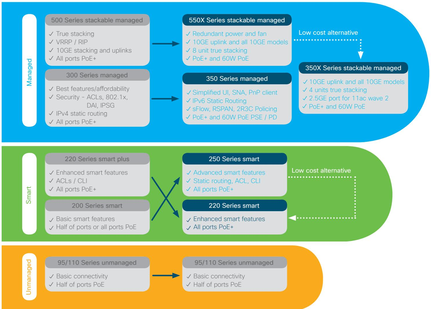
The new portfolio includes 550X, 350X, 350 and 250 Series switches to replace the current 500, 300 and 200 Series. There is no change to 220 Series smart switches and 110 and 95 Series unmanaged switches. They will continue to be integral parts of the Cisco SMB switching portfolio.
